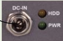
DC Power Input Connector with Screw Lock
